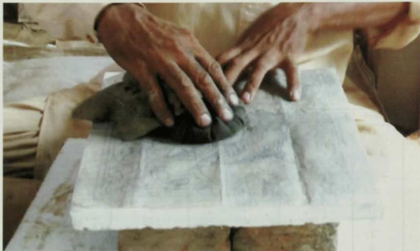
Pl. 54 Transferring of design on tile.
