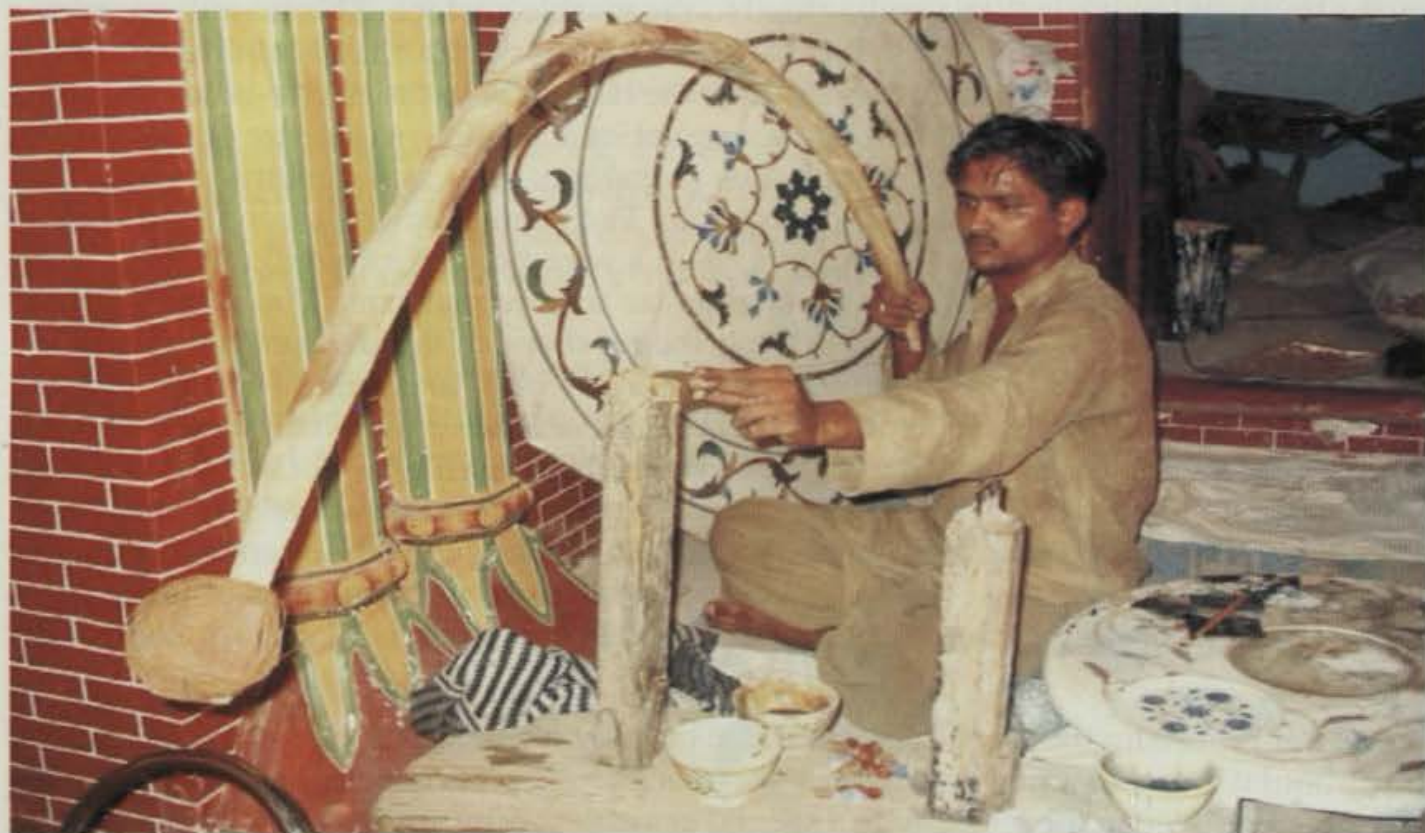
Pl. 96. Cutting of semi precious stone with wire bow
