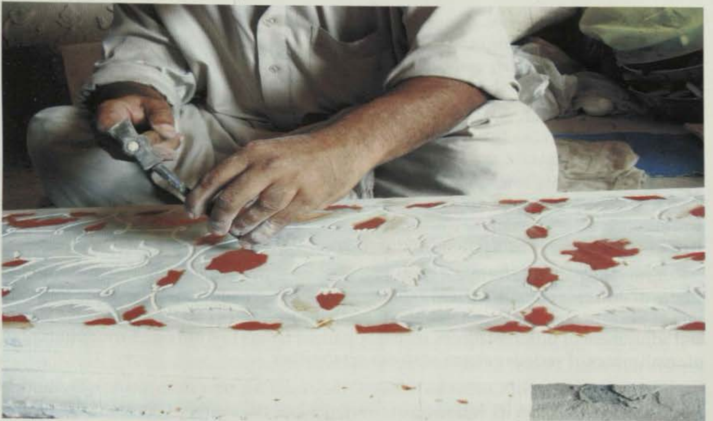
Pl. 98 Engraving in marble for fixing semi-precious stones
