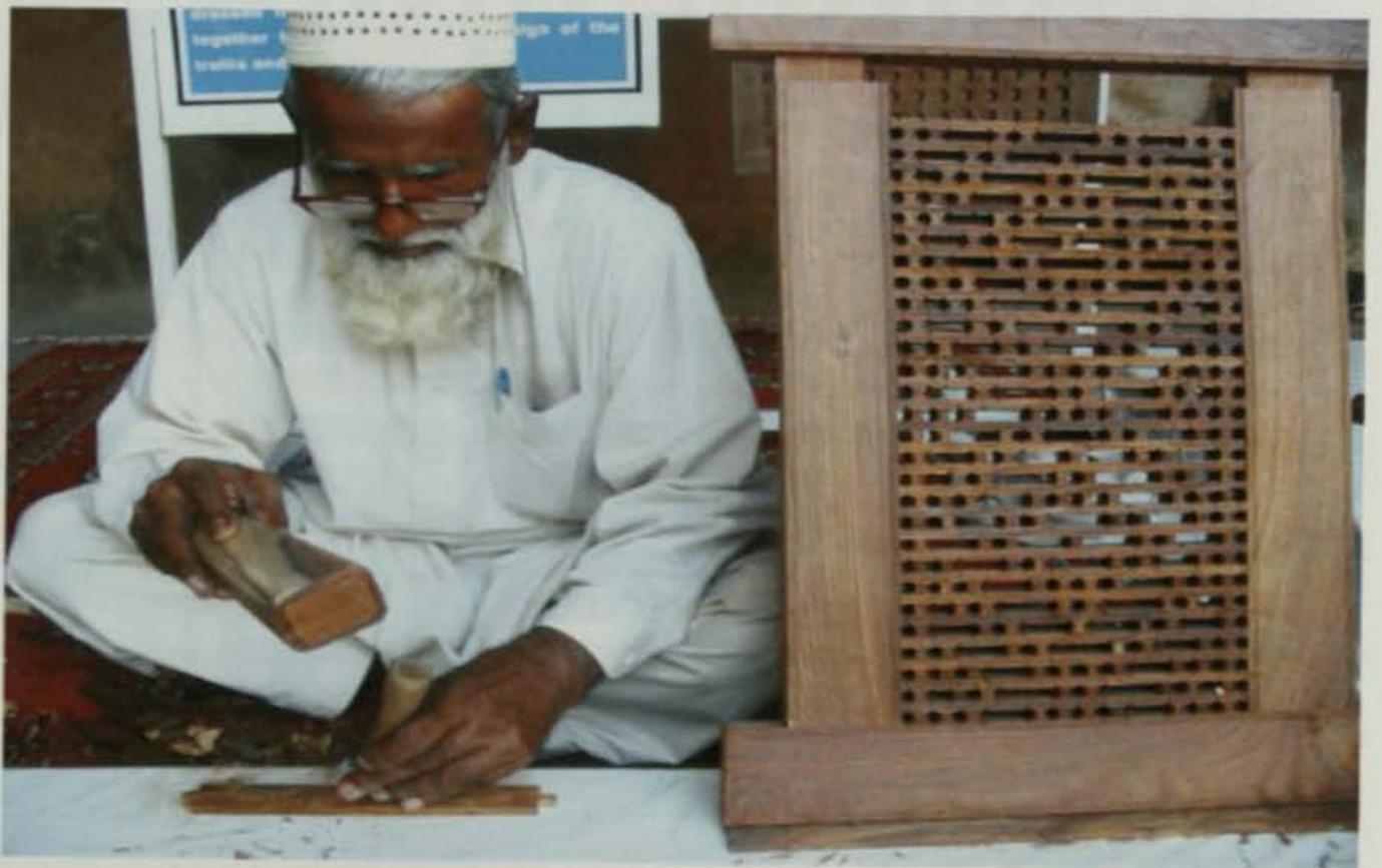
Pl. 110 Manufacturing of lattice wood work.
