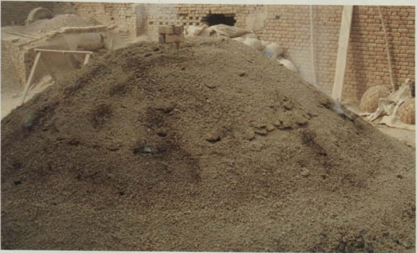
Pl. 128 Burning of kankar for kankar lime in shape of heap.
